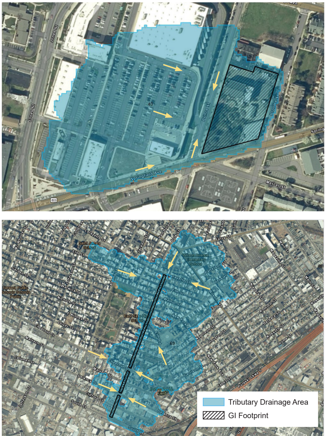
Figure 2.5 | Examples of Tributary Drainage Area Delineations
